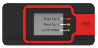
LEDs code below corresponds to the system and Inview S during normal operation.
